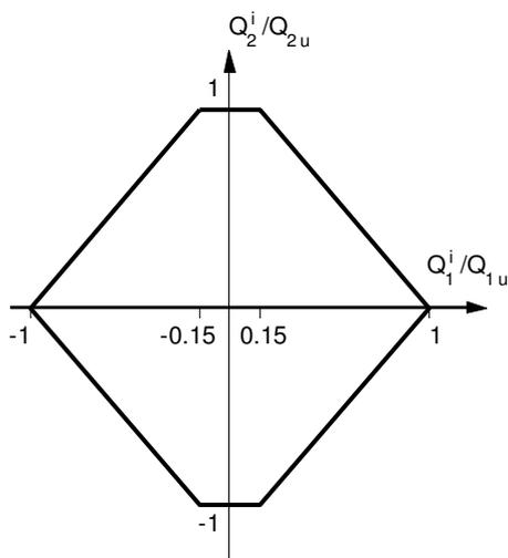
Fig 2. Piecewise linear hexagonal yield model.
