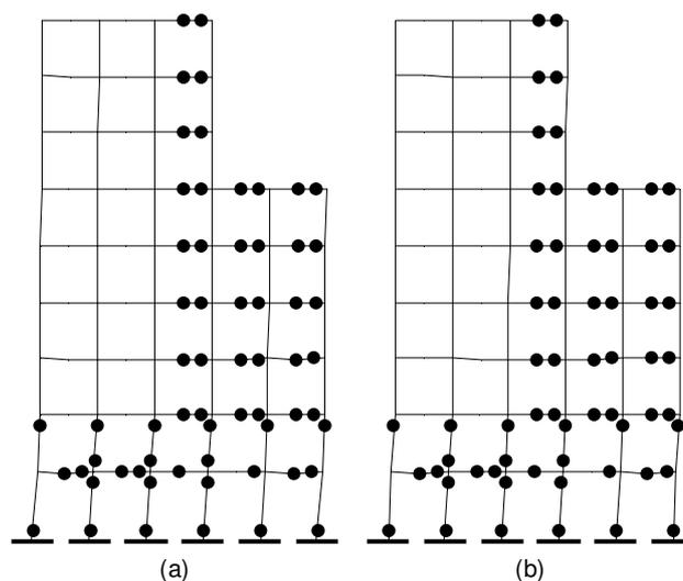
Fig 3. Collapse mechanisms (a) maximum collapse limit and (b) minimum collapse limit; • denotes plastic hinge.
