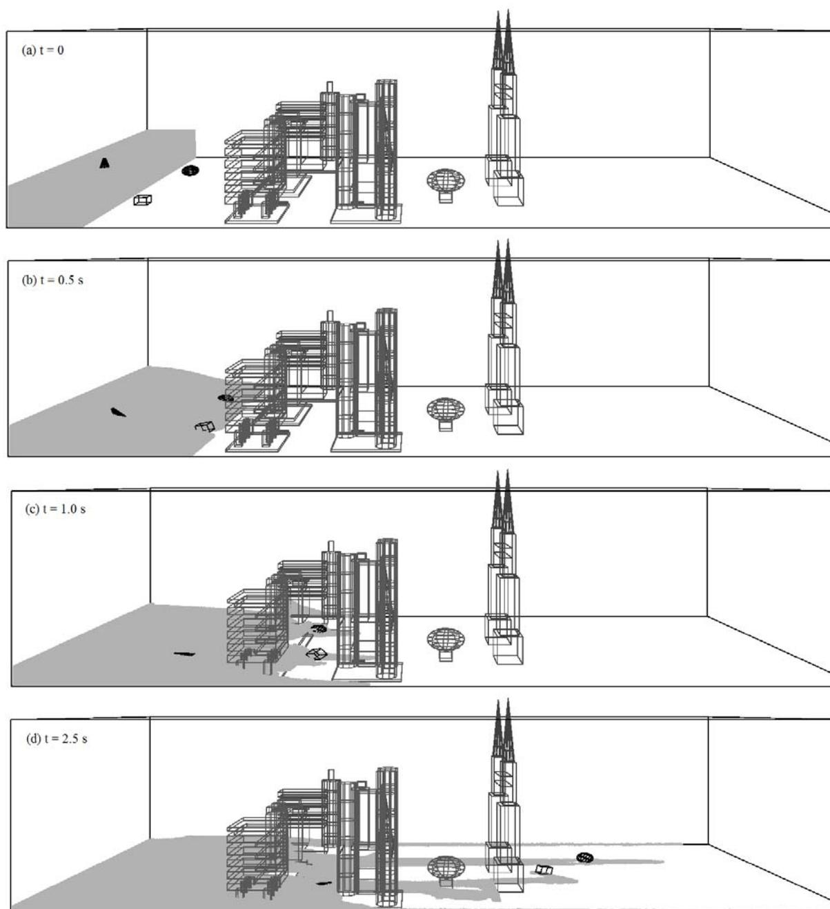
Fig. 5 Displacement of flooding flow and floating objects computed by SPH model ( $t = 0, 0.5, 1.0, 2.5$  s)
