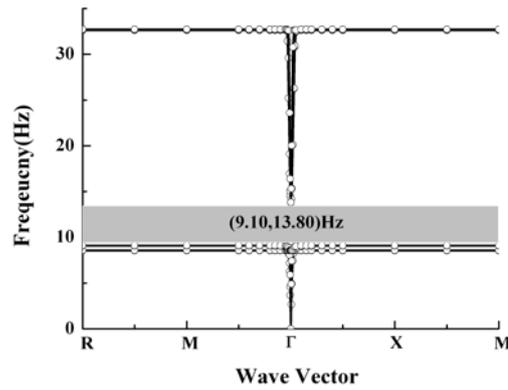
Fig. 7. Dispersion relationship of a coated cube inclusion periodic structure with  $a=1.0\text{m}$   $b=0.6\text{m}$ , and  $t=0.1\text{m}$
