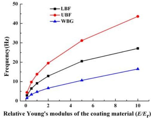
Fig. 12. Influences of the Young's modulus of the coating material on the first band gap
