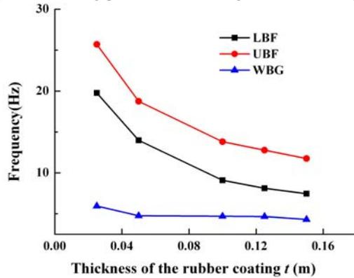
Fig. 10. First band gap as a function of  $t$ , the thickness of the rubber coating
