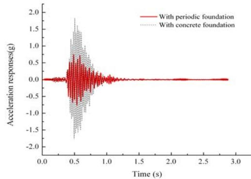
Fig. 4. Horizontal acceleration responses at the tops of the frames under the modified 1984 Bishop earthquake [12]
