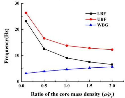
Fig. 13. First band gap versus the mass density of the core material
