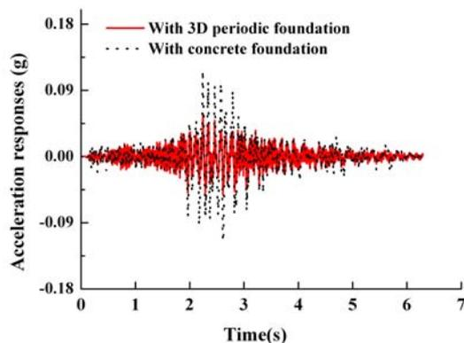
Fig. 17. Acceleration responses for the lumped mass node in vertical direction under the 1984 Bishop MCG-UP seismic record
