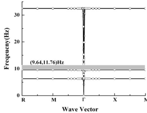
Fig. 8. Dispersion relationship of a coated sphere inclusion periodic structure with  $a=1.0\text{m}$   $d=0.6\text{m}$ , and  $t=0.1\text{m}$
