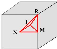
Fig. 6. First irreducible Brillouin zone of periodic structures
