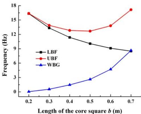
Fig. 11. First band gap as a function of  $b$ , the side length of the square core lowered as the thickness of the rubber coating increases. Different with Fig.6, the WBG changes small in this case.
