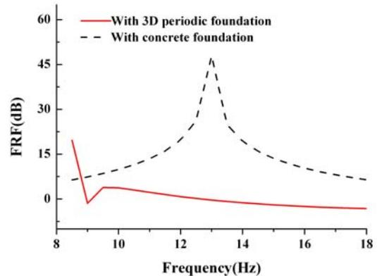
Fig. 16. Displacement frequency responses function for the lumped mass node in horizontal direction
