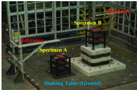
Fig.1 Test setup for one-dimensional periodic foundation
