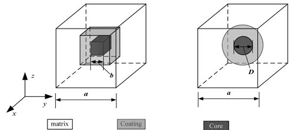
Fig. 5. Illustration of the unit cell of a three-dimensional periodic foundation
