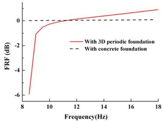
Fig. 15. Displacement frequency responses function of the lumped mass node in vertical direction
