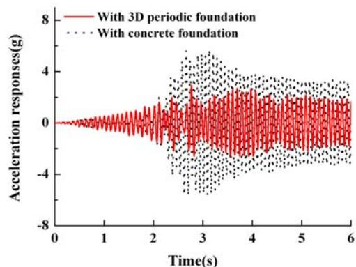
Fig. 18. Acceleration responses for the lumped mass node in horizontal direction under the 1984 Bishop MCG360 seismic record
