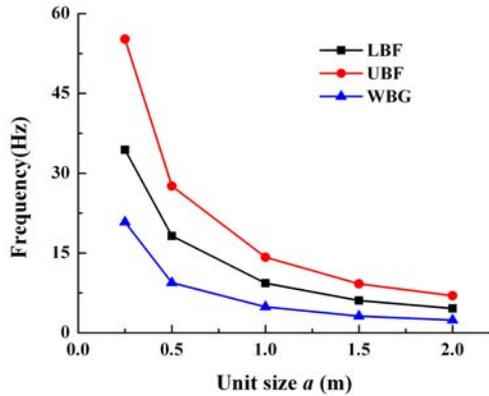
Fig. 9. First band gaps versus the side length of the unit cell ( $a$ )
