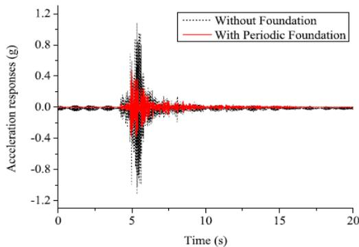
Fig. 2. Horizontal acceleration responses at the tops of the frames under the 1975 Oroville earthquake [9]
