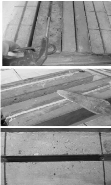
Fig.3. Strengthening of test specimens
