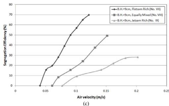
Fig. 3. Segregation efficiency versus inlet air velocity in different mixture compositions for bed height of a) 4cm, b) 6cm, c) 9cm
