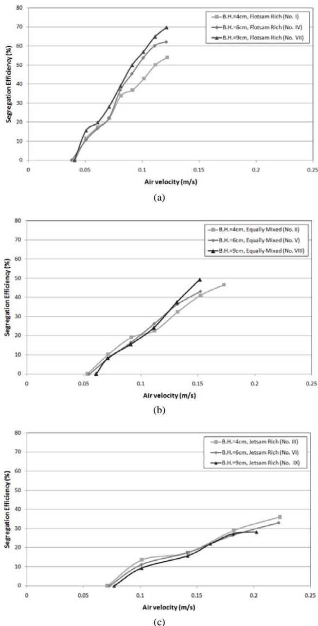
Fig. 4. Segregation efficiency versus inlet air velocity in different bed heights for mixture compositions of a) Flotsam-rich, b) Equally mixed, c) Jetsam-rich
