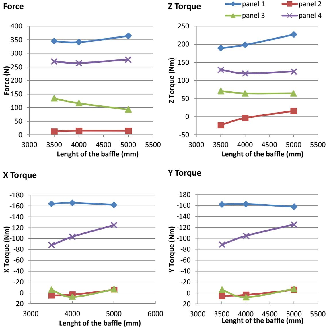
Fig. 4: Force and torque (related to the center of the panel) on the solar panels at the different positions. Distance between protection panel and solar field: 10 m.
