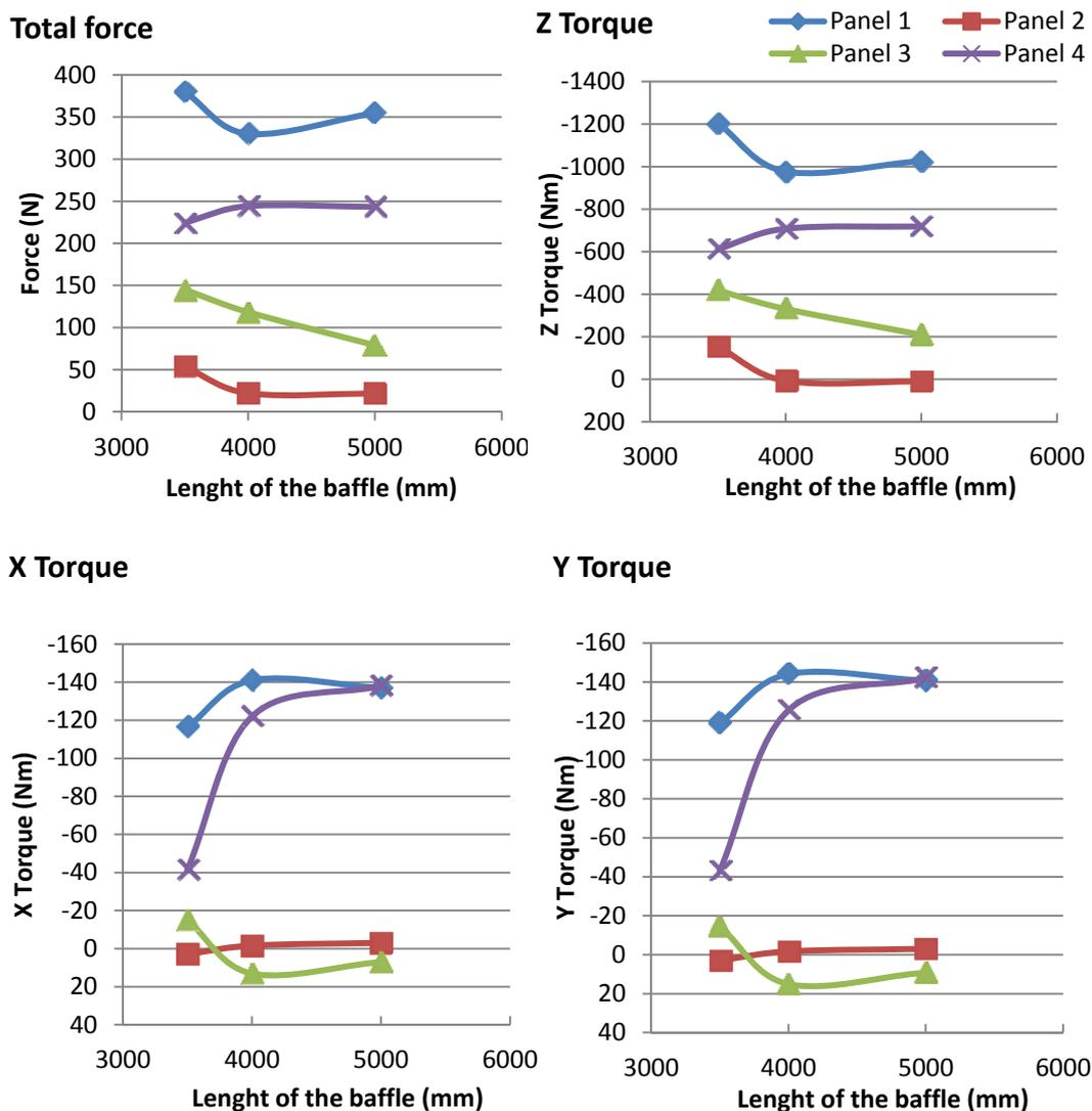
Fig. 4: Force and torque (related to the center of the solar panel) on the solar panels at the different positions. Distance between protection panel and solar field: 15 m.
