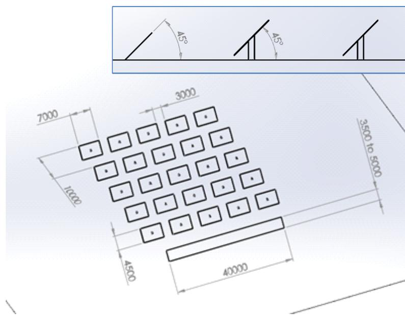
Fig. 1: The array of solar panels: dimensions (mm). On top: lateral view.
