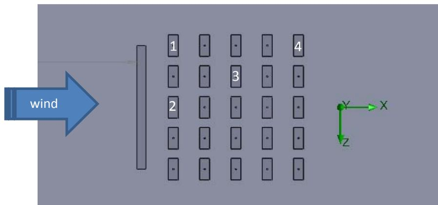
Fig. 2: The array of solar panels and the positions tested.
