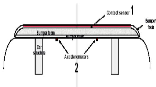
Fig 3 Position of sensors in bumper (1: contact sensor, 2: accelerometers).
