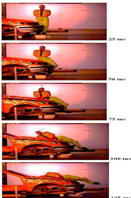
Fig 6 Crash test in 40 km/h with a pedestrian dummy and an active bonnet
