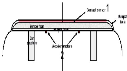
Fig 3 Position of sensors in bumper (1: contact sensor, 2: accelerometers).
