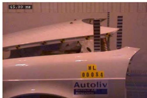
Fig 4 Bonnet with protection system in activated (lifted) position.
