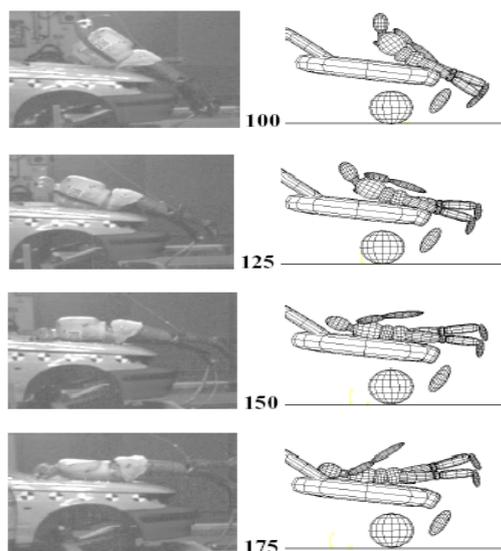
Fig 5 the comparison of the kinematics of the pedestrian dummy with a MADYMO model (at 30 km/h and at centre-line).
