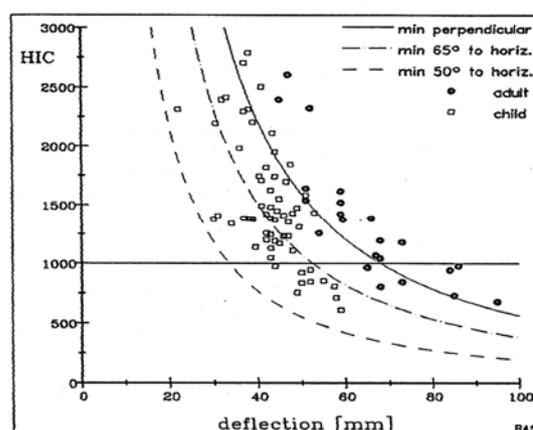
Fig 1 Bonnet head form tests performed at 40 km/h impact speed.
