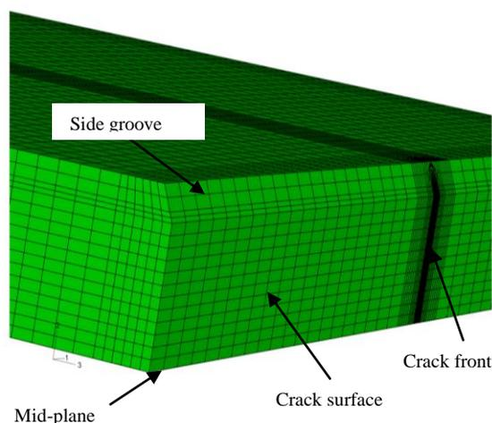
Fig. 2. Finite element model for a side grooved specimen.
