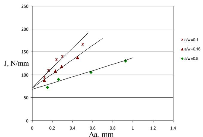
Fig. 6 The fracture resistance curve ( $J-\Delta a$  curve) for deep and shallow cracked specimens  $a/w=0.5, 0.16$  and  $0.1$ ,  $B/w=0.5$ .
