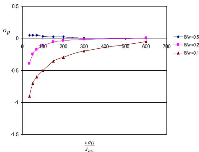
Fig. 3 Out-of-plane effect as a function of deformation levels for deeply cracked geometries  $a/w=0.5$  with different thickness ratios  $B/w$ .
