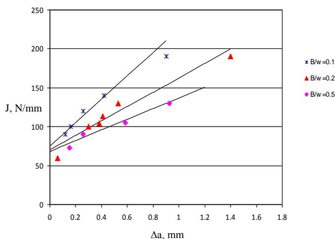
Fig. 5 The fracture resistance curve ( $J-\Delta a$  curve) for thick and thin single edge notched bend specimens with  $a/w=0.5$  and  $B/w=0.5, 0.2$  and  $0.1$ .
