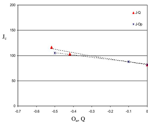
Fig. 7 A comparison between J-Op and J-Q locus ( $J_c$  at  $\Delta a=0.2\text{mm}$ ).
