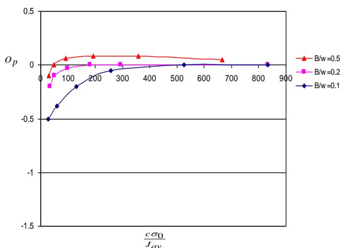
Fig. 4 Out-of-plane effect as a function of deformation levels for shallow cracked geometries  $a/w=0.1$  with different thickness ratios  $B/w$ .
