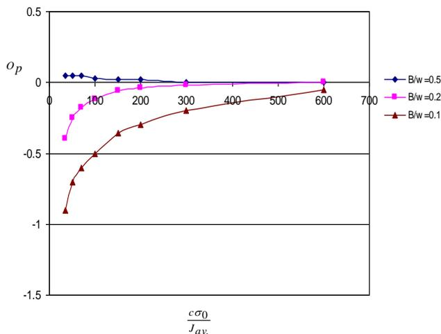
Fig. 3 Out-of-plane effect as a function of deformation levels for deeply cracked geometries  $a/w=0.5$  with different thickness ratios  $B/w$ .
