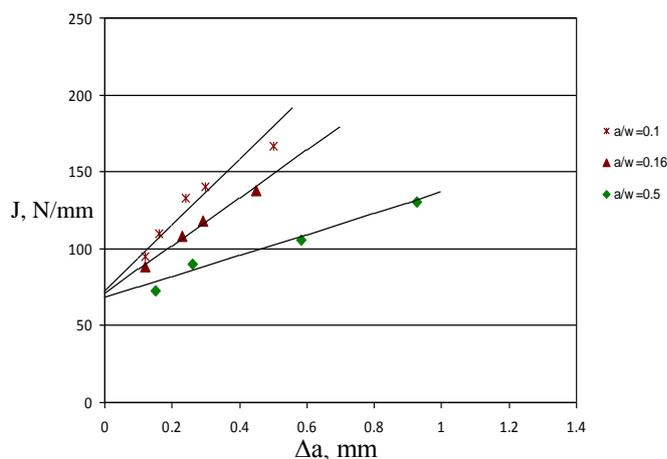
Fig. 6 The fracture resistance curve ( $J-\Delta a$  curve) for deep and shallow cracked specimens  $a/w=0.5, 0.16$  and  $0.1$ ,  $B/w=0.5$ .
