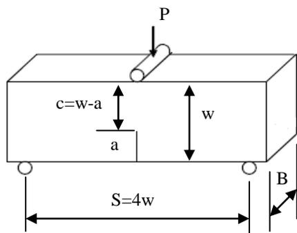
Fig. 1. A standard single edge cracked bend specimen.
