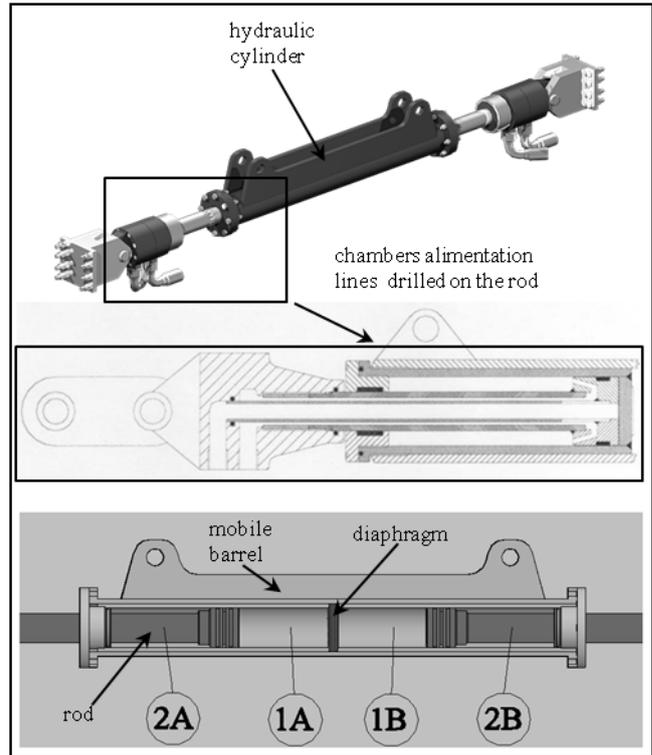
Fig. 3. Hydraulic cylinder details.
