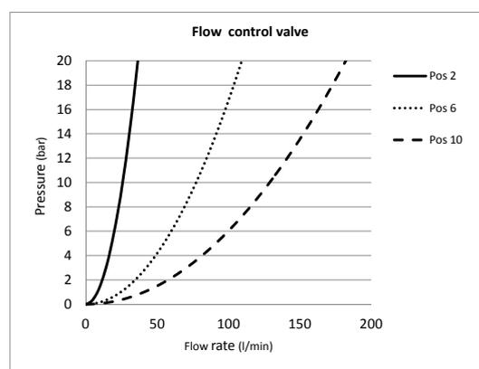
Fig. 7. Flow control valve characteristics.
