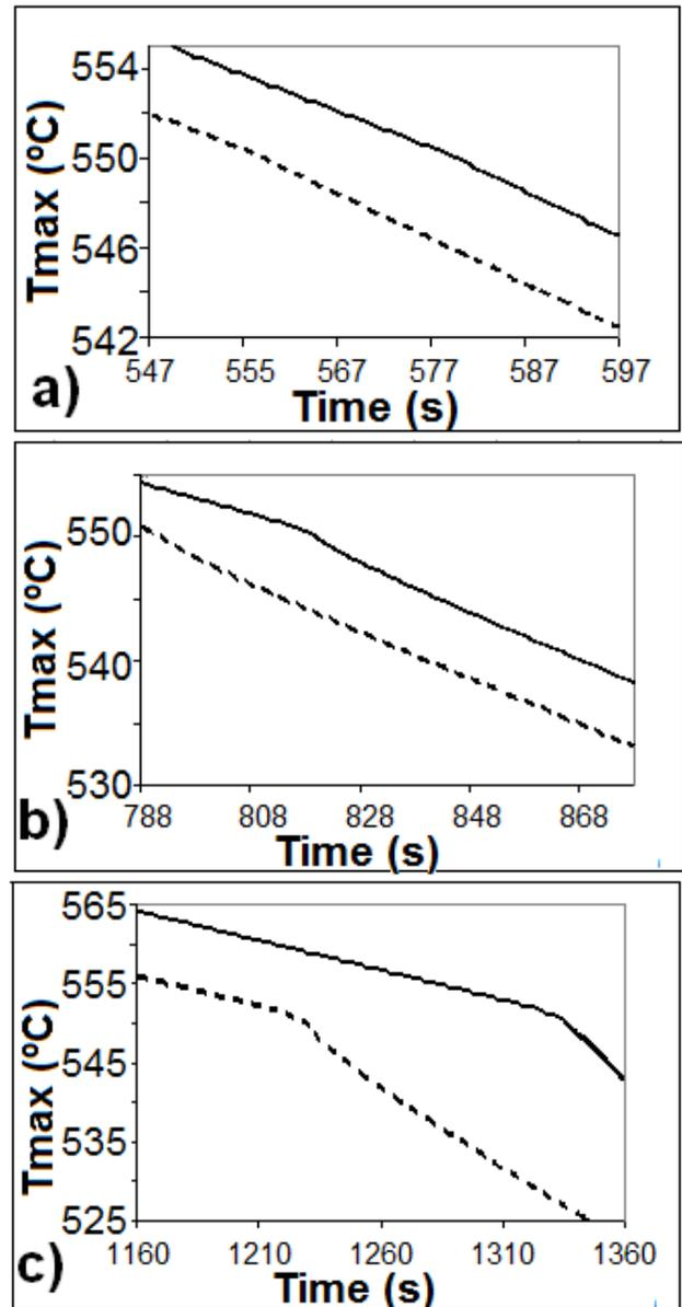
Fig. 2. Evolution of maximum temperatures for Newtonian and pseudo plastic fluid for three aspect ratios: a) R=1.33, b) R=1.77, c) R=2.
