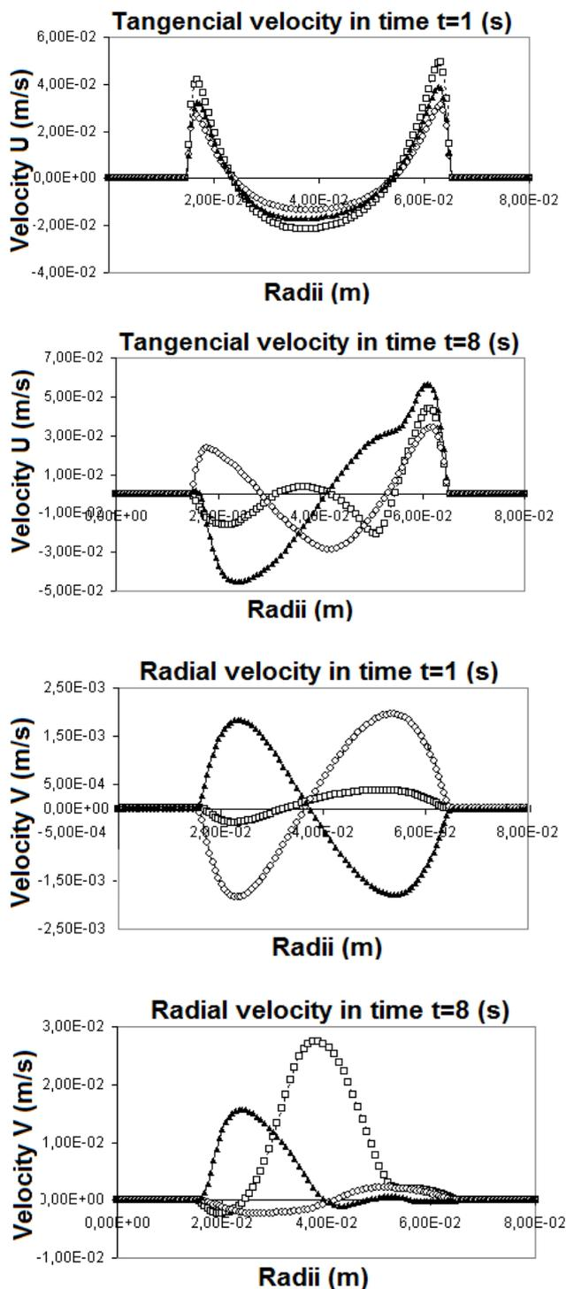
Fig. 3. Tangential and radial velocity in annular solidification for  $R=1.77$  and  $Ra=8.69 \times 10^{10}$ .
