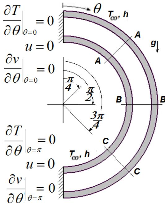
Fig. 1. Alloy annular cylindrical solidification in a graphite mold.
