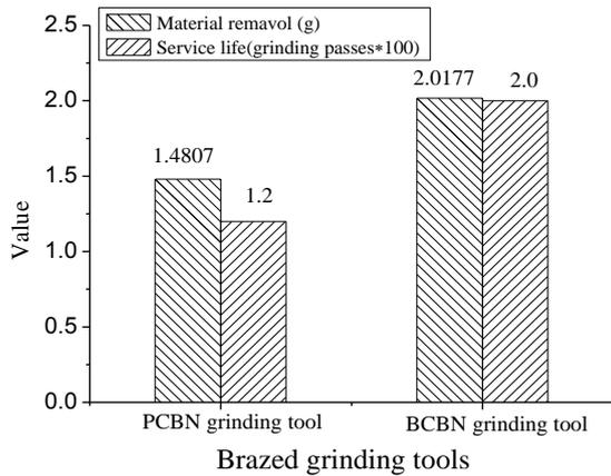
Fig. 6 The comparison of grinding performance of BCBN and PCBN grinding tools
