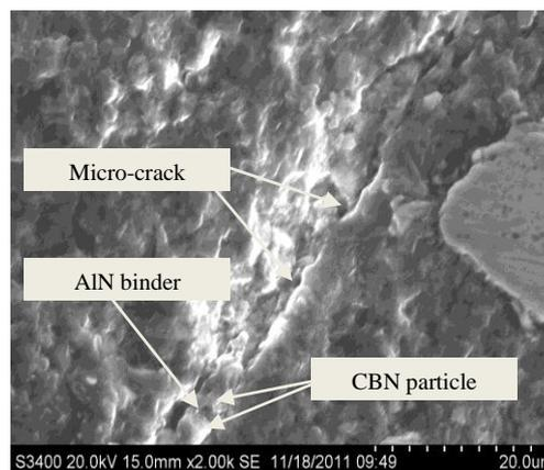
Fig. 5 Micro-crack path of PCBN grain
