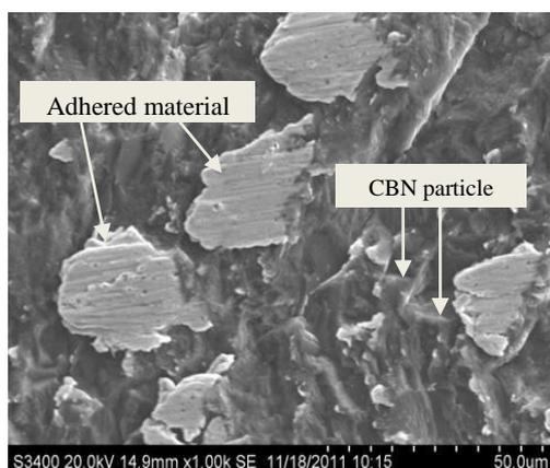
Fig. 4 Micro-fracture topography of BCBN grain
