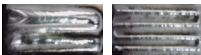
(a) Distorted weld bead using high current and lower torch speed (b) Thin weld bead at lower current & higher torch speed Fig. 4. Weld sizes from different process parameter
