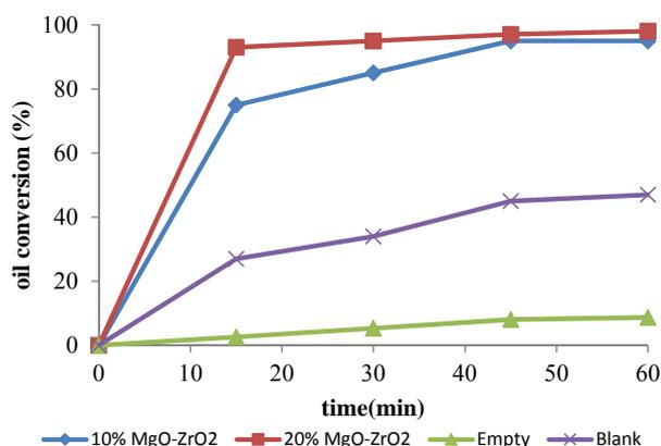
Fig. 5. Waste oil conversion to biodiesel at 225°C as function of time in the absence of catalyst, over blank ZrO<sub>2</sub> support, 10%MgO/ZrO<sub>2</sub> and 20%MgO/ZrO<sub>2</sub> respectively (alcohol to oil molar ratio 18:1, catalyst amount 3 wt.%).
