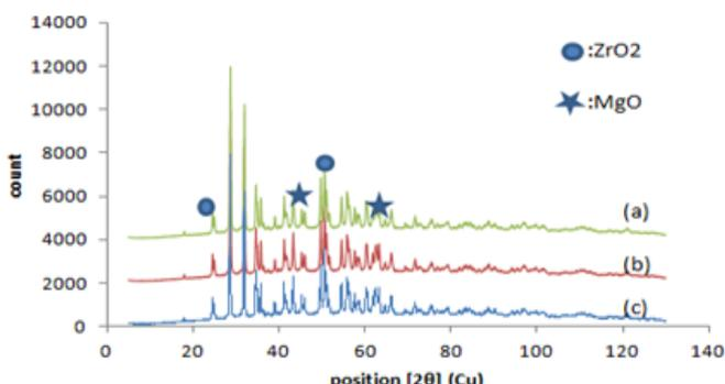
Fig. 3. XRD pattern of calcined MgO/ZrO<sub>2</sub> (a) before reaction; (b) after transesterification reaction at  $150^\circ\text{C}$  and (c) after transesterification reaction at  $225^\circ\text{C}$
