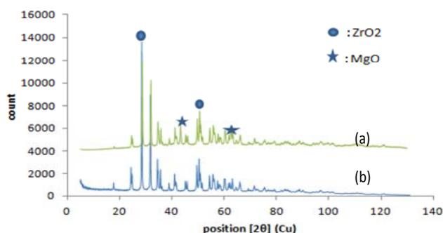
Fig. 2. XRD pattern of (a) 20% calcined MgO/ZrO<sub>2</sub>, (b) calcined blank ZrO<sub>2</sub>
