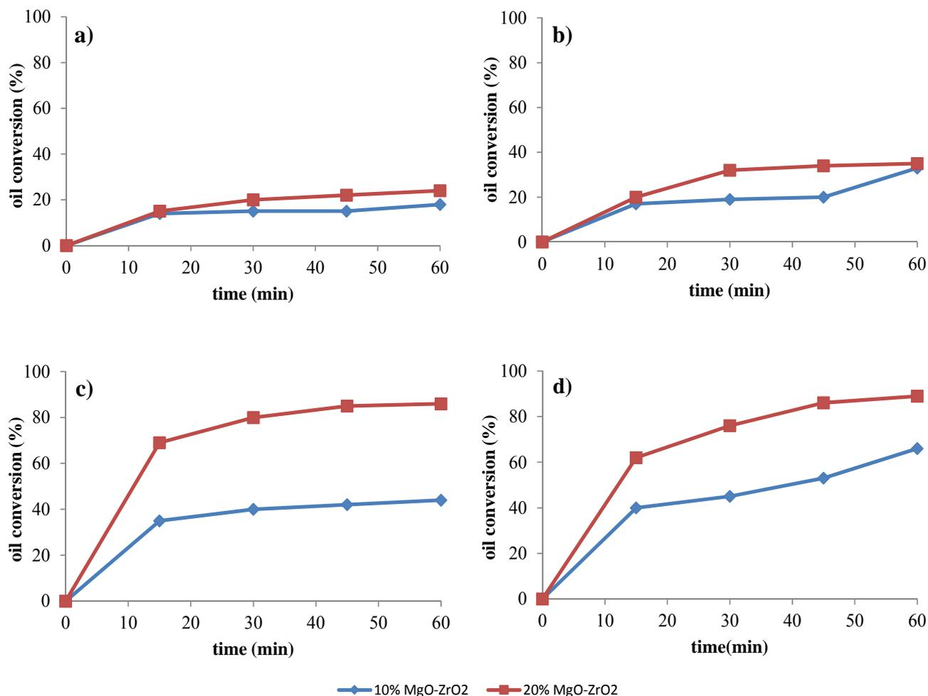
Fig. 4. Effect of temperature: a) 60°C, b) 150°C, c) 175°C and d) 200°C, time (0 to 60 min) and  $MgO$  loading (10 and 20% $MgO$ ) on waste oil conversion to biodiesel (catalyst amount 3wt.%)
