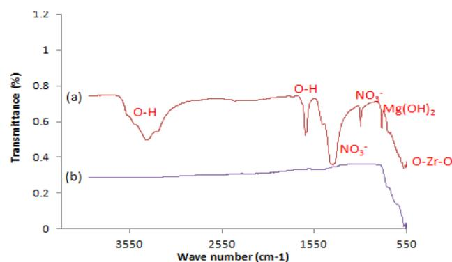
Fig. 1. FTIR spectrum of (a) dried catalyst ; (b) 20% calcined MgO/ZrO<sub>2</sub>
