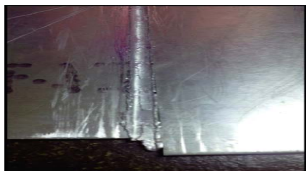
(d). Defect formed due to larger welding of 4 mm diameter tool is used
