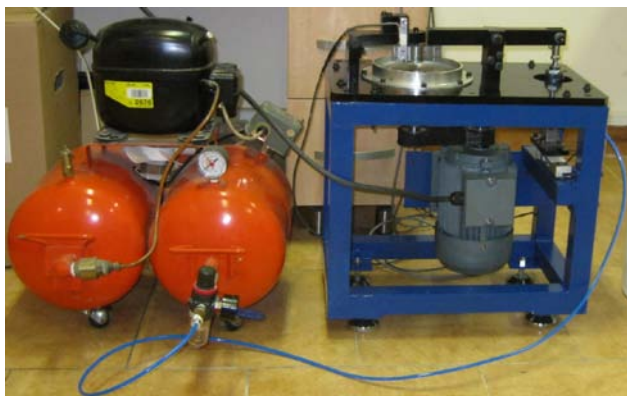
Fig. 2. Setup of the cryogenic wear test simulator used in this research
