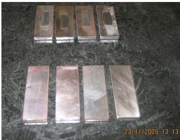
Figure. 1 Standard test specimen of size 75×26×6 mm
