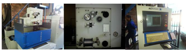
Fig. 4. (a) WEDM machine (b) wire reel (c) Actspark control console
