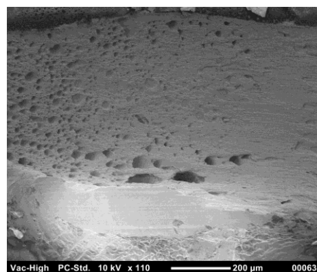
Fig. 7. Fracture surface of 1812 capacitor after 15 years of simulated field time.
