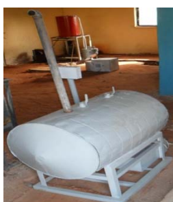
Fig 6: The fabricated fire-tub boiler
