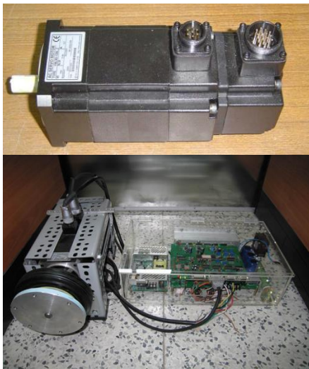
Figure 3. Entity diagram (a) YBL9D-130L (b) drive control panel.
