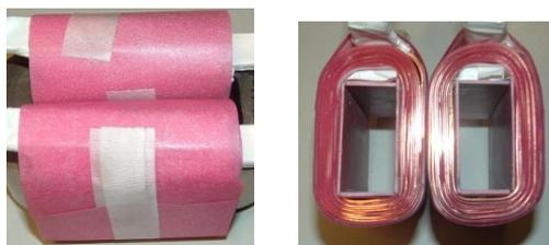
Fig. 6. 7 layers copper foil of thickness 0.7mm separated by interleaving insulation of 0.125mm
