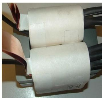
Fig. 8a. Foil wound HF transformer
