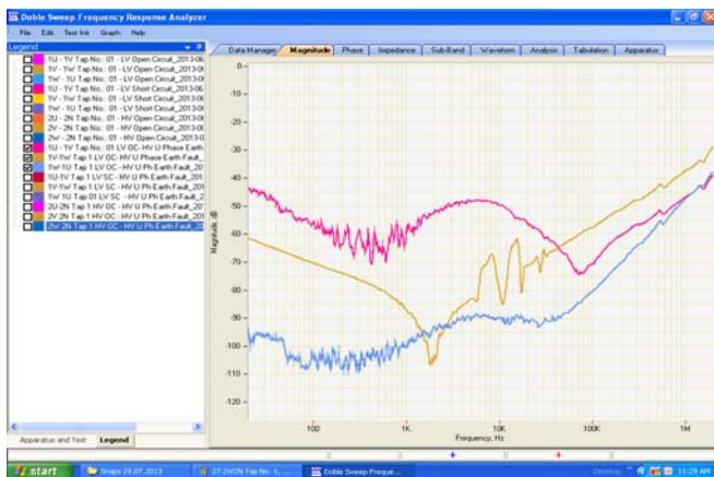
Fig. 5 HV LV Open - 1U Earth Fault
