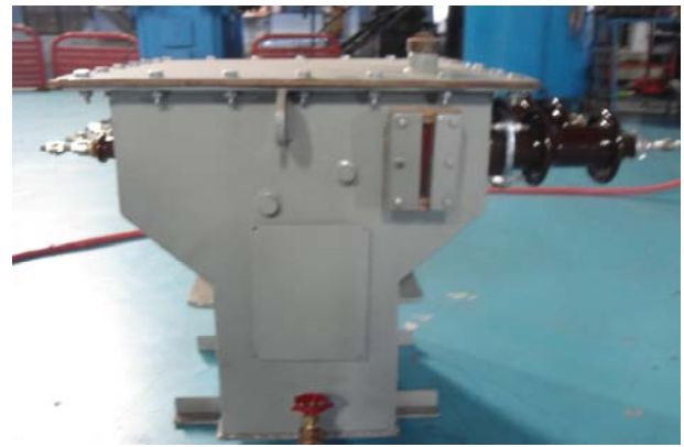
Fig. 1 10 KVA, 11000 V/440 V, 3-phase, 50 Hz, Dyn11 Power Transformer
