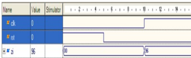
Fig. 10. VHDL simulation of the BBS generator module.
