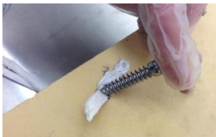
Fig 2. The specimen was fixed with a metallic round-head interference screw (Arthrex Inc, Naples, FL) into the foam block
