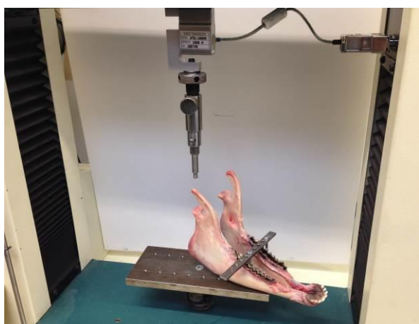
Fig 3. The mounted specimen in a Hounsfield testing machine. The specimen was mounted into the machine using a custom made fixture.
