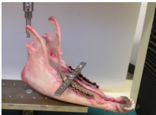
Fig 2. The sheep jaw bone sample was mounted into the testing machine
