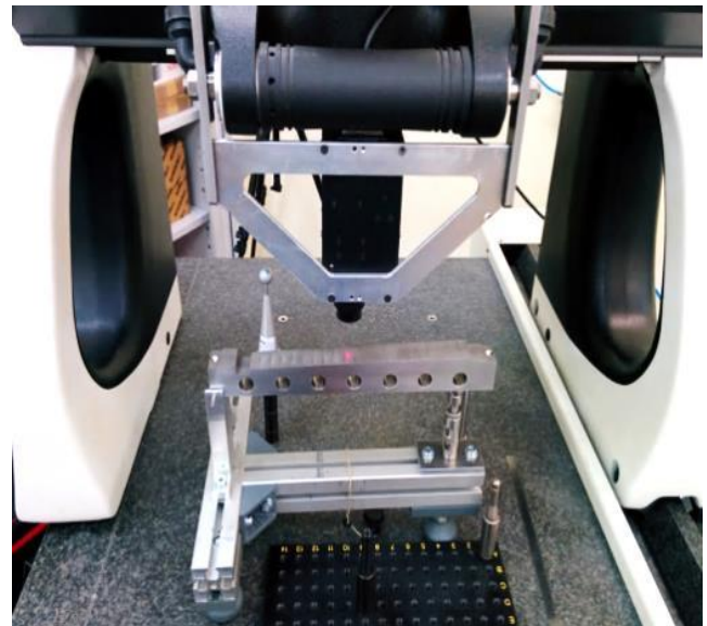
Fig. 1. Conoscopic holography digitizing of test specimen.
