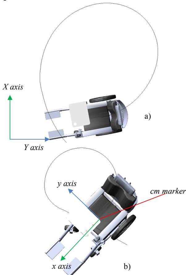
Fig.8. Wheelchair trajectory: combined motion (a) and steering motion (b).
