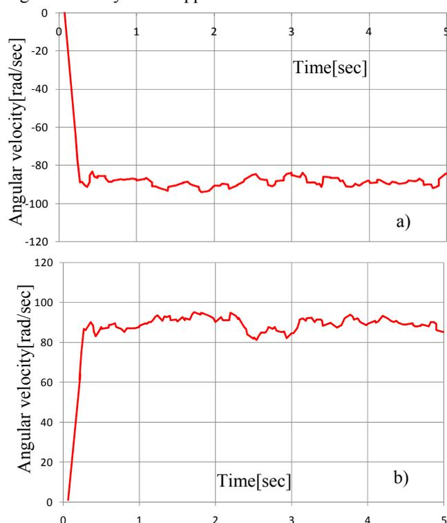
Fig.11. Right and left wheel angular velocity, in case of steering simulation.
