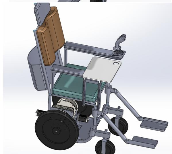
Fig.4. Wheelchair assembly model in Solid Works.
