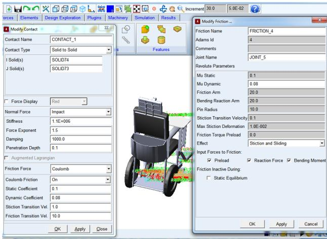
Fig.7. Wheelchair contact and friction parameters.
