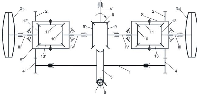
Fig.1. Kinematics scheme of wheelchair transmission.
