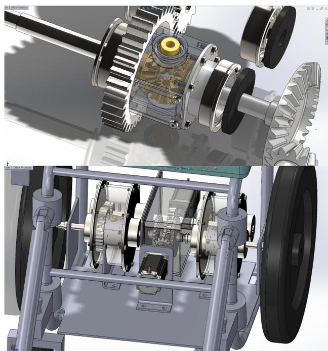
Fig.3. Wheelchair transmission assembly in Solid Works.
