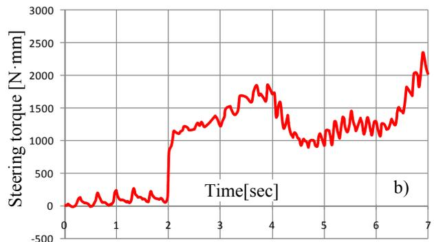
Fig.10. Traction and steering torque variation, in case of combined motion.
