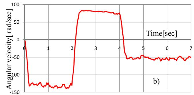
Fig.9. Right and left wheel angular velocity, in case of combined motion.
