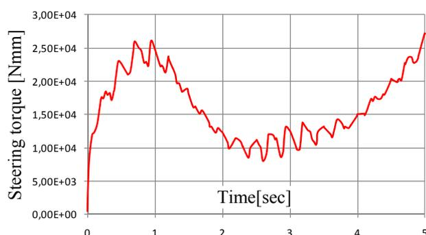
Fig.12. Steering torque variation, in case of steering simulation.
