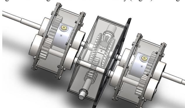
Fig.2. CAD model of differential transmission.
