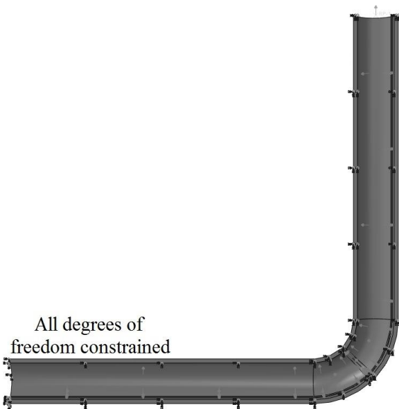
Fig. 3. Half symmetric model with boundary and loading conditions.
