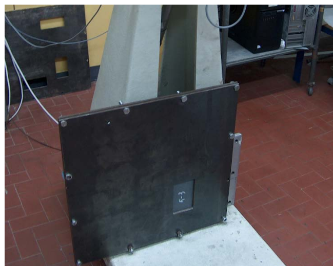
Fig. 2. Modified Charpy impact test machine.
