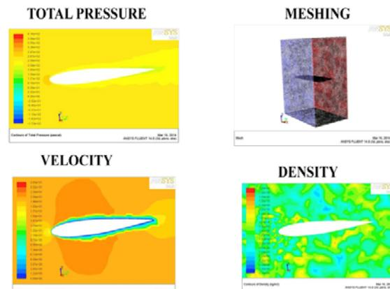
Fig 4: Contours of wing without winglet
