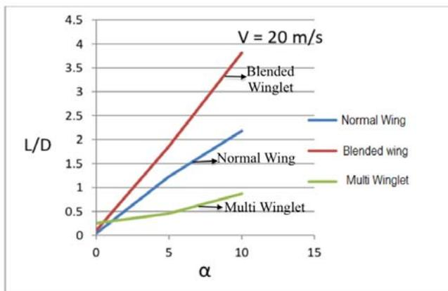
Fig 11: Graphical comparison (experimental) of wings L/D Vs  $\alpha$  at 20m/s
