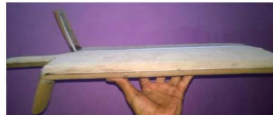
Fig3: NACA0015 wing with multi winglets
