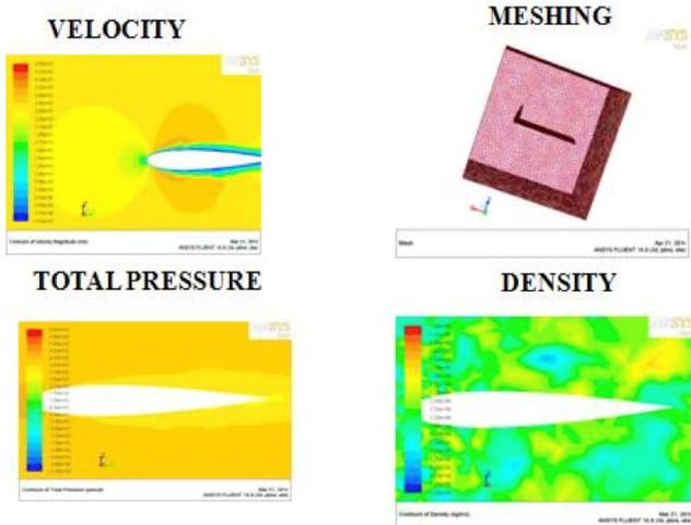
Fig 5: Contours of wing with blended winglet
