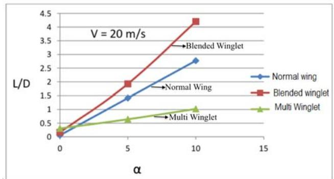
Fig 8: Graphical comparison (theoretical) of wings L/D Vs  $\alpha$  at 20m/s
