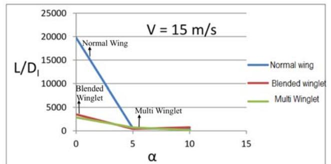
Fig 9: Graphical comparison of wings L/D<sub>1</sub> Vs  $\alpha$  at 15m/s
