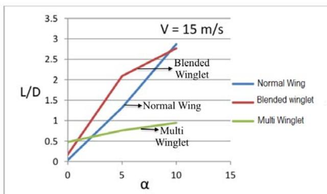
Fig 12: Graphical comparison (experimental) of wings L/D Vs  $\alpha$  at 15m/s
