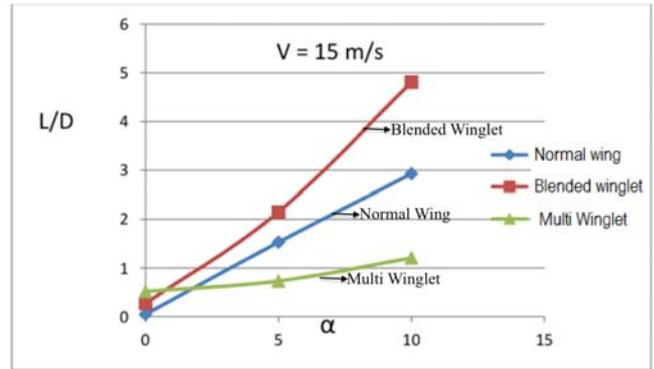
Fig 7: Graphical comparison (theoretical) of wings L/D Vs  $\alpha$  at 15m/s
