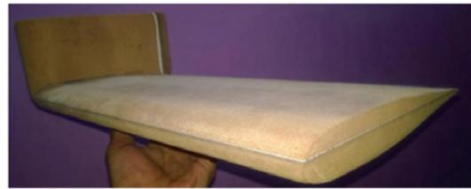
Fig 2: NACA0015 wing with blended winglet
