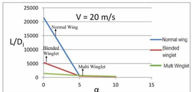
Fig 10: Graphical comparison of wings L/D<sub>1</sub> Vs  $\alpha$  at 20m/s
