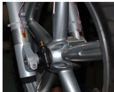
Fig. 9. Fork sliders instrumented with strain gauge.
