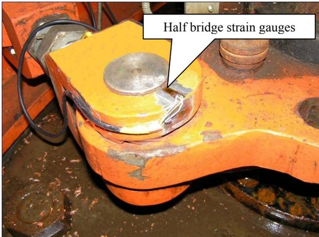
Fig. 1. The H4450-23 pitchfork with half bridge strain gauges
