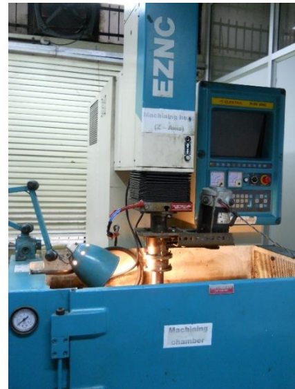
Figure 3: EDM with rotary tool set-up
