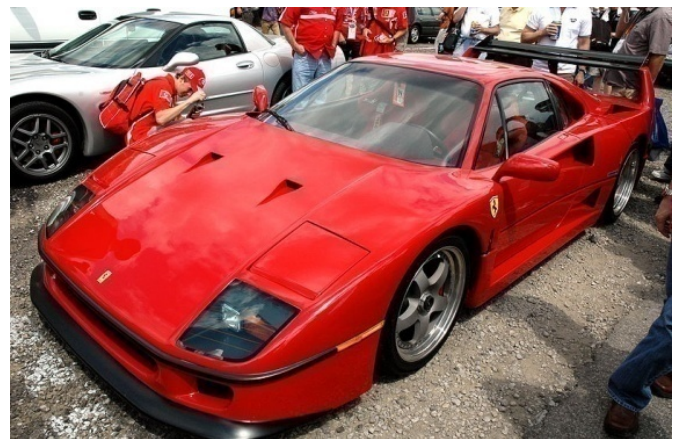
Fig.1. NACA Flush inlets on racing car
