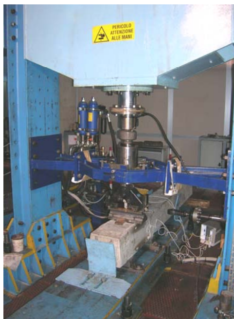
Fig. 12. Layout for rail under static test and strain gages readings.
