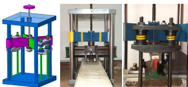
Fig. 7. Plant for impact tests on rail fastenings.
