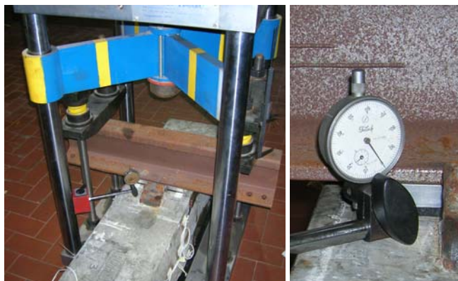
Fig. 11. Initial positioning and resetting of comparators.
