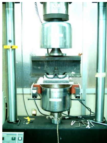
Fig. 9. Test arrangement and laser disposition during the vertical stiffness test.
