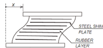
Fig.1. Elastomeric steel-reinforced isolator
