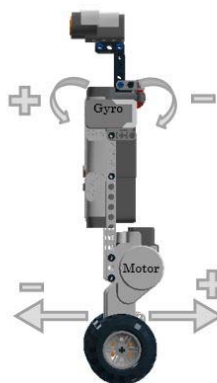
Fig.9. Direction of wheels’ rotation according to body lean.
