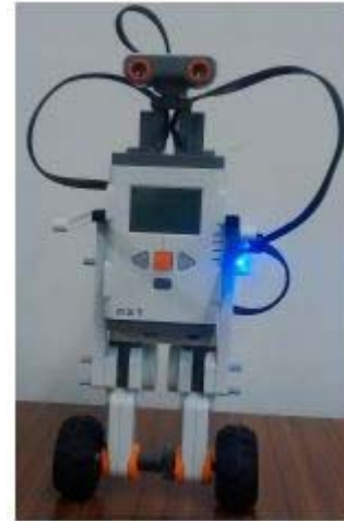
Fig.1. Configuration of the Equilibrist Lego Robot.
