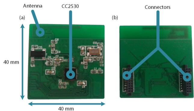
Fig. 3. Developed CC2530 board with integrated PCB antenna: (a) Top view; (b) Bottom view.
