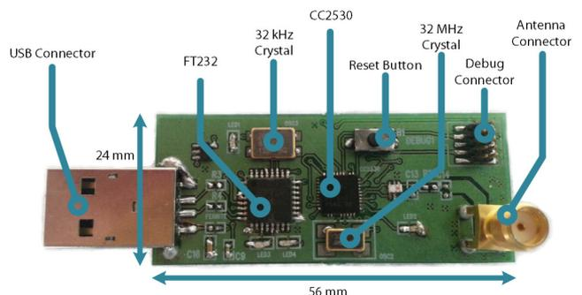
Fig. 4. Developed base station board.
