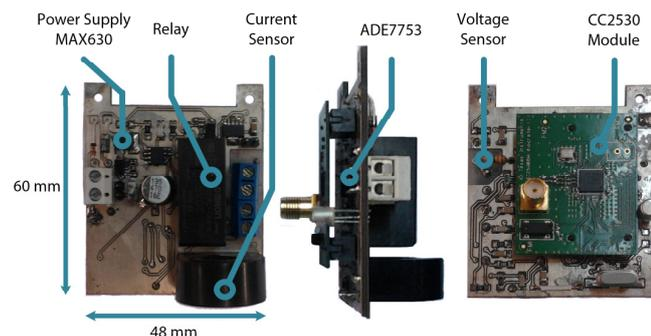
Fig. 2. Top, side and bottom views of the developed sensor node board.
