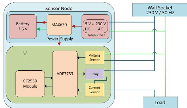
Fig. 1. Block diagram of the sensor node hardware.
