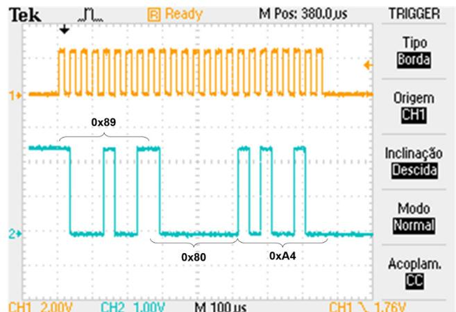
Fig. 8. SPI communication between the CC2530 and the ADE7753.
