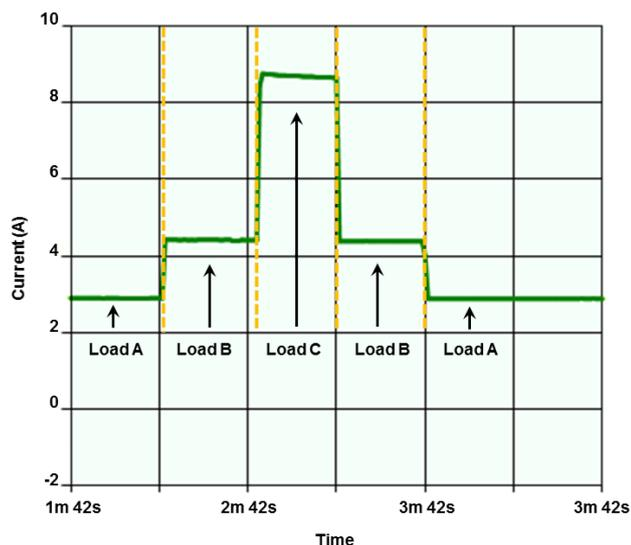
Fig. 9. RMS value of the current for different loads.
