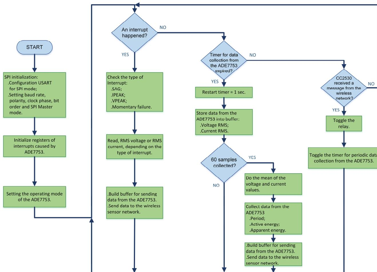
Fig. 5. Flowchart of the application developed for the CC2530 sensor node.
