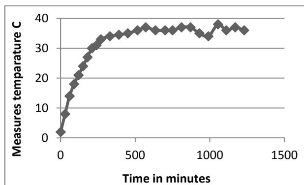
Fig. 8. Temperature rise of the windings at the open circuit test
