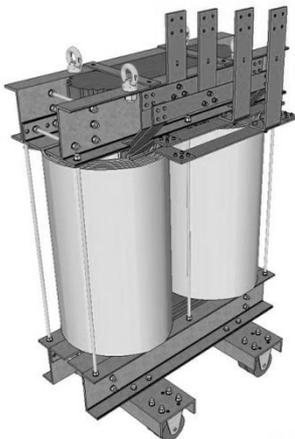
Fig. 2. Three dimensional model of the 1.2MVA transformer
