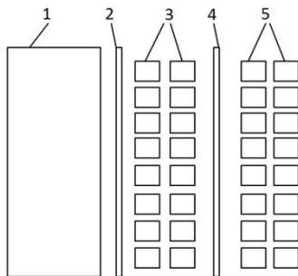
Fig. 1. Simplified diagram of a transformer coil structure . 1. Si-Steel core, 2. Primary winding to core insulation barrier, 3. Primary winding 4. Primary winding to Secondary winding insulation barrier, 5. Secondary winding; note: Depending on the design specific conditions designers use air ducts in between any of the above layers.
