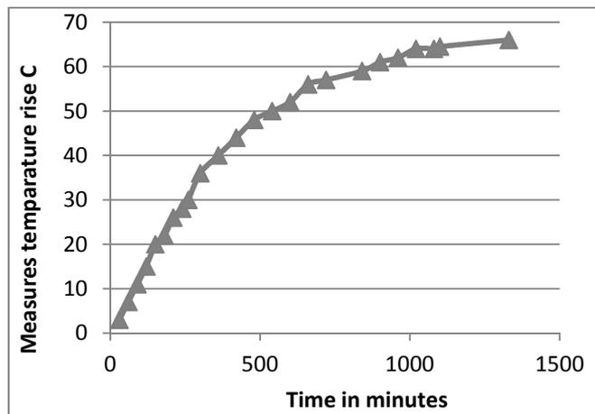
Fig. 7. Temperature rise of the core at the open circuit test
