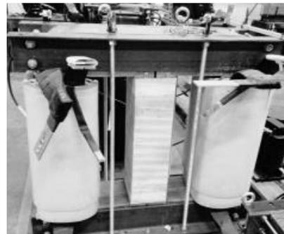
Fig. 6. 90kVA open delta phase conversion transformer
