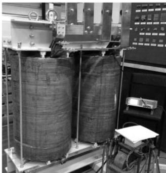
Fig. 5. 1.2MVA transformer testing arrangement
