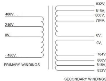
Fig. 3. Transformer schematic diagram
