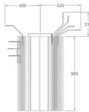
Fig. 4. Construction of one of the two coils
