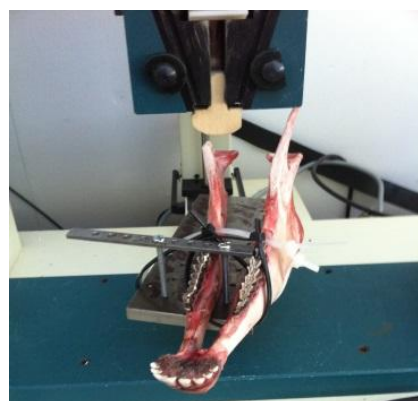
Fig 2. The sheep jaw bone sample mounted into the testing machine
