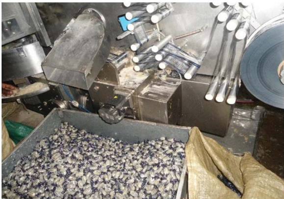
Fig 2 Typical automated manufacturing sweet wrapping machine
