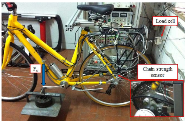
Fig. 2. Experimental setup for the estimation of the torque acting on the pedal starting from the chain strength sensor.
