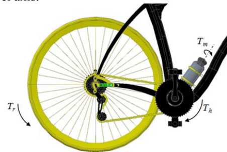
Fig. 4. Scheme of the pedelec drive system.
