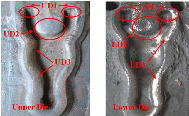
Fig 5 Inspection of damage on the actual blocker dies (a) upper die and (b) lower die
