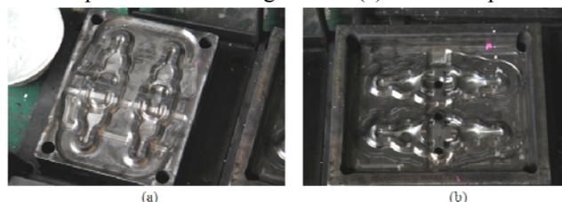
Fig 2 New blocker dies (a) upper die; (b) lower die
