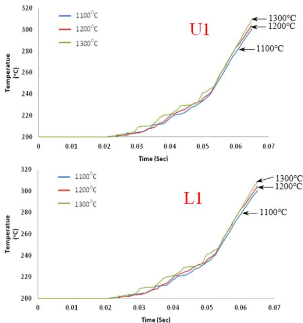
Fig 13 Die temperature during forging at location U1 and L1; initial billet temperature of 1100°C, 1200°C and 1300°C
