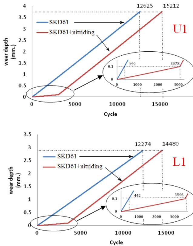
Fig 19 Wear depth variation with no. of cycles for SKD61 compared to SKD61 with nitriding treatment
