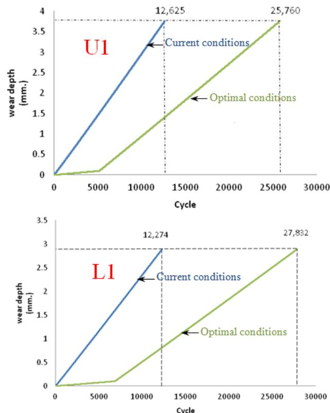
Fig 20 Comparison of die life for current conditions and optimal conditions; (a) upper die and (b) lower die
