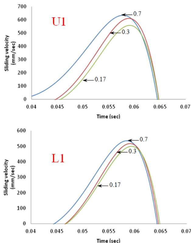
Fig 16 Sliding velocity during forging at location U1 and L1; coefficient of friction of 0.17, 0.3 and 0.7
