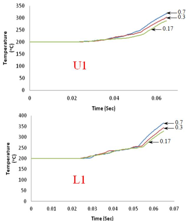
Fig 17 Die temperature during forging at location U1 and L1; coefficient of friction of 0.17, 0.3 and 0.7
