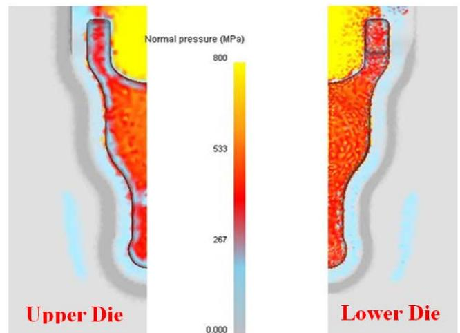
Fig 8 Normal pressure on upper and lower dies
