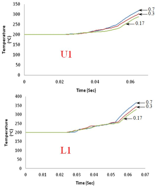
Fig 17 Die temperature during forging at location U1 and L1; coefficient of friction of 0.17, 0.3 and 0.7
