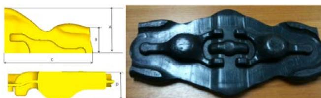
Fig 4 FE results and actual forged part with dimensional comparison
