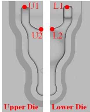
Fig 10 Locations where wear is calculated and measured
