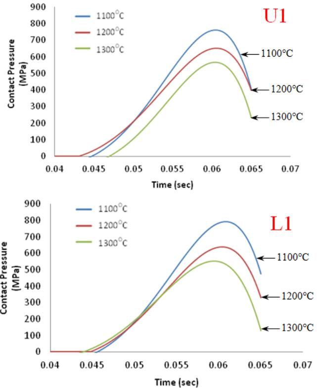
Fig 11 Contact pressure during forging at location U1 and L1; initial billet temperature of 1100°C, 1200°C and 1300°C
