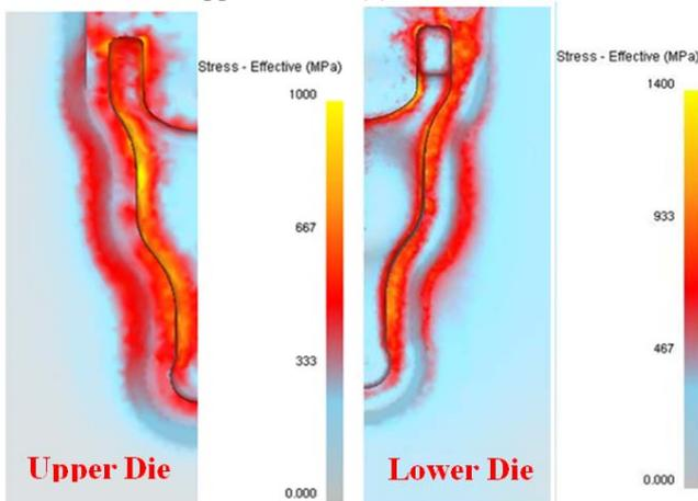
Fig 6 Effective stresses on upper and lower dies
