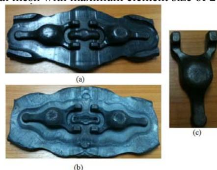
Fig 1 (a) forged workpiece after blocker die; (b) forged workpiece after finishing die and (c) final workpiece
