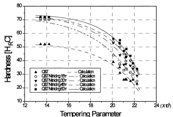
Fig 9 Material hardness as a function of tempering parameter [10,11]
