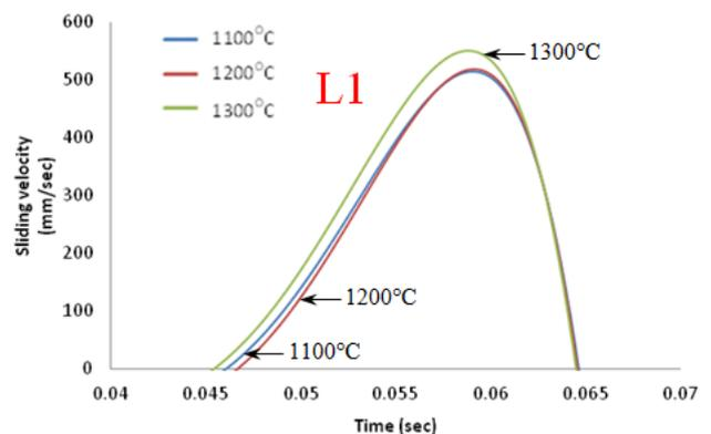
Fig 12 sliding velocity during forging at location U1 and L1; initial billet temperature of 1100°C, 1200°C and 1300°C
