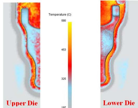
Fig 7 Temperature distribution on upper and lower dies
