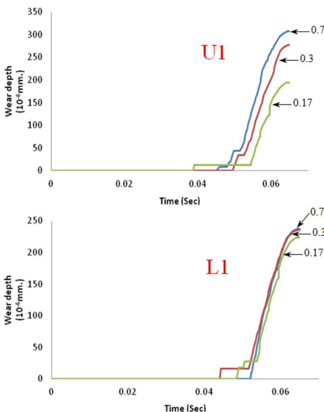
Fig 18 wear depth per cycle during forging at location U1 and L1; coefficient of friction of 0.17, 0.3 and 0.7
