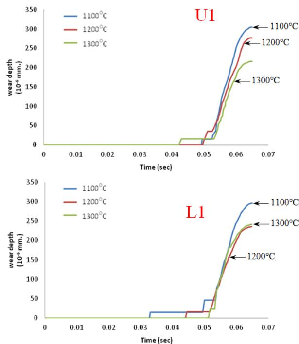
Fig 14 Wear depth per cycle during forging at location U1 and L1; initial billet temperature of 1100°C, 1200°C and 1300°C
