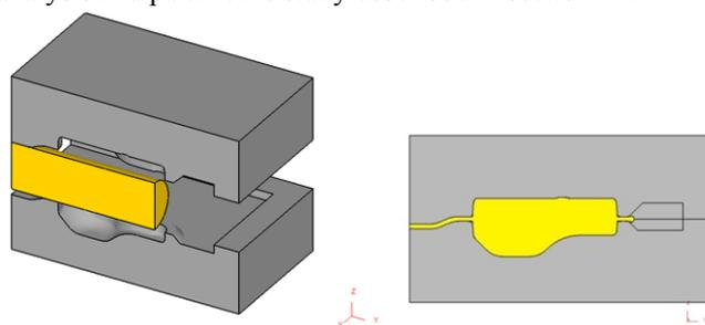
Fig 3 Finite element model of forging process
