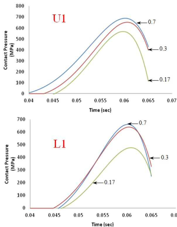
Fig 15 Contact pressure during forging at location U1 and L1; coefficient of friction of 0.17, 0.3 and 0.7
