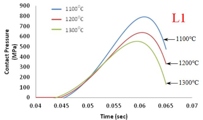
Fig 11 Contact pressure during forging at location U1 and L1; initial billet temperature of 1100°C, 1200°C and 1300°C
