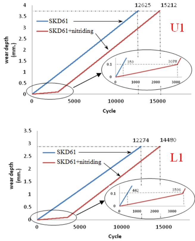
Fig 19 Wear depth variation with no. of cycles for SKD61 compared to SKD61 with nitriding treatment
