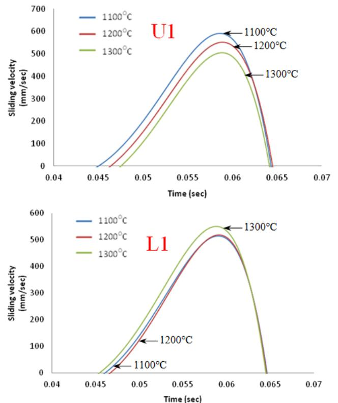
Fig 12 sliding velocity during forging at location U1 and L1; initial billet temperature of 1100°C, 1200°C and 1300°C
