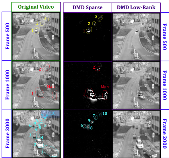
Fig. 2. Demonstration of the foreground/background separation of videos using the DMD algorithm. The example problem is motivated by a surveillance problem which tries to identify moving cars and pedestrians from stationary/parked cars in a video feed.
