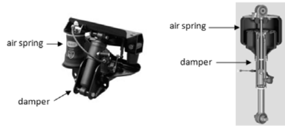
Fig 8. Integrated air springs and damper.
