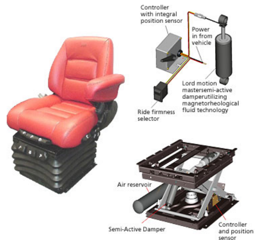
Fig. 2. Example of cabin-to-seat (by SEARS) semi-active suspension systems.
