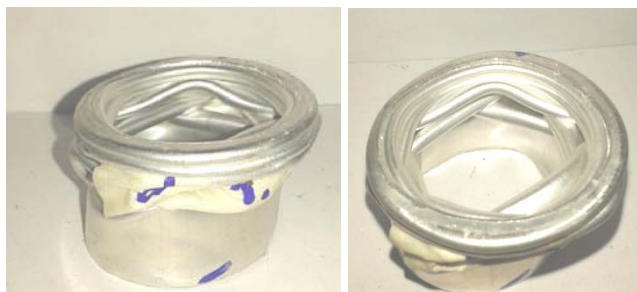
Fig. 9. Final mode of AL tube.
