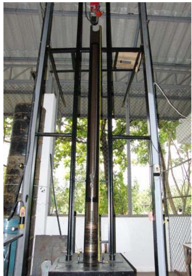
Fig. 3. Vertical impact testing machine
