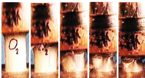
Fig. 5. Progressive collapse of AL/GFRP - 2 Layers and [0 2 ]
