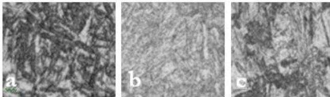
Fig. 8 - Micrographs of the center of the HAZ: (a) without pre and post-heat treatment; (b) Only pre-heating; (c) pre and post-heating.
