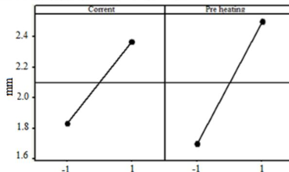
Fig 4 – Main effect on the penetration in millimeter.
