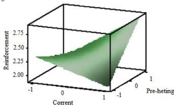
Fig. 7 - interaction current x pre heating
