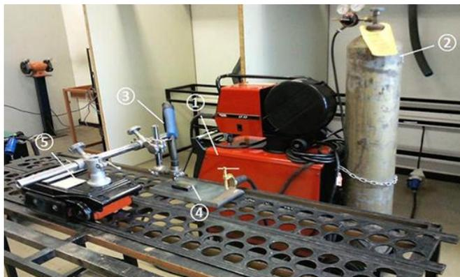
Fig.2. welding tests. 1) power supply; 2) shielding gas; 3) torch; 4) specimen; 5) mechanized movement system
