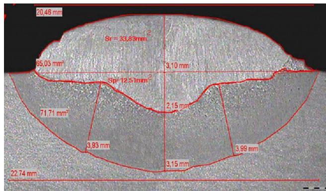
Fig. 3 - specimen photo with demarcation of areas and linear measurements
