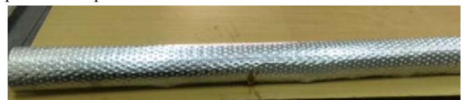
Fig. 3 Photographic view of protruded tube ( x/d=10 and y/d=10 )
