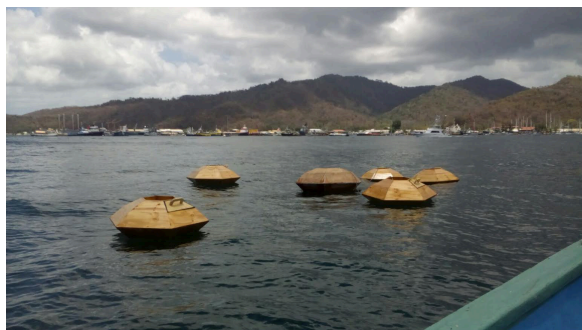
Fig. 3. Wave Energy Converter (WEC) array test in Crews Inn Bay, Trinidad.
