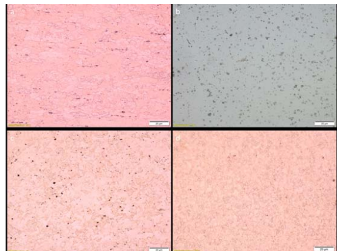
Fig 3: Microstructural images at 50x magnification using the optical microscope showing (a) Cu parent material (b) Al parent material (c) Cu Heat affected zone (HAZ) (d) Cu Thermo-mechanically affected zone (TMAZ)
